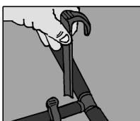
11. Now secure the 13mm poly tube by pushing Hold Down Stakes into the soil at regular intervals along the tube.
