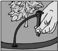
9. Push the Asta PC Drip Spike into the soil near the plant so that the water will wet the rootzone effectively. Install further Asta PC Drip Spikes until you have completed the installation according to your plan.
