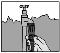
regulator & connect the 13mm poly tube onto TIP: It is easier to push the tube onto fittings if you CAREFULLY dip the end of the tube into a container of hot water for a few seconds.
