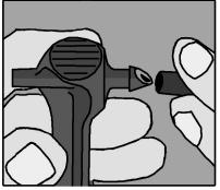
8. Cut the 4mm tube to a suitable length and push the free end of the uPVC tube onto the barbed side of the Asta PC Drip Spike..
