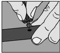
7. Push other end of the adaptor into the hole in the 13mm poly tube.
