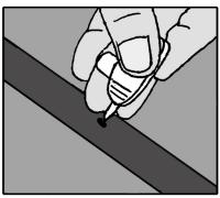
5. Using the Key Punch supplied, make a hole in the 13mm poly tube where you want an emitter to be placed.
