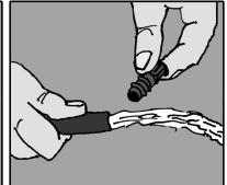
12. Before you install the End Plugs to seal the ends of the 13mm poly tube, turn on the tap & flush out any pieces of plastic or soil . Turn off the tap and insert the End Plugs.
